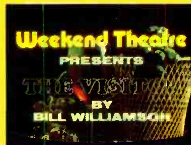
KEY OUTPUTS R.G.B and keying outputs are supplied from the Marquee-2000 so the output may be downstream keyed with the surrounding or drop shadow edging.
